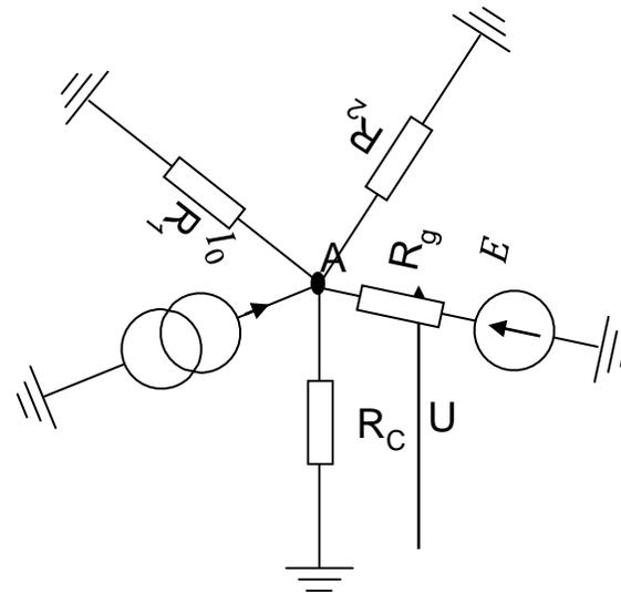
$$V_A = \frac{\frac{E}{R_g} + I_0}{\frac{1}{R_1} + \frac{1}{R_2} + \frac{1}{R_g} + \frac{1}{R_C}}$$
