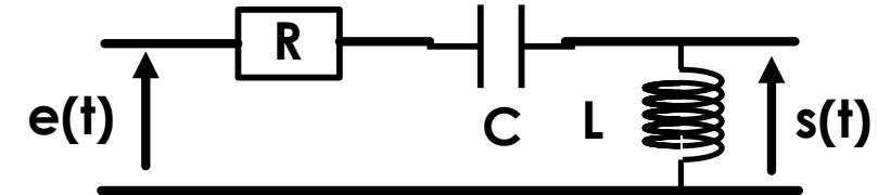
$$\Phi(\omega) = \pi - \arctan \left( \frac{2m}{\frac{\omega_0}{\omega} - \frac{\omega}{\omega_0}} \right)$$
