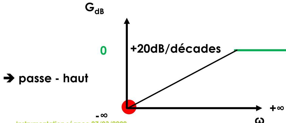
$$\Phi(\omega) = \frac{\pi}{2} - \arctan \left( \frac{\omega}{\omega_0} \right)$$
