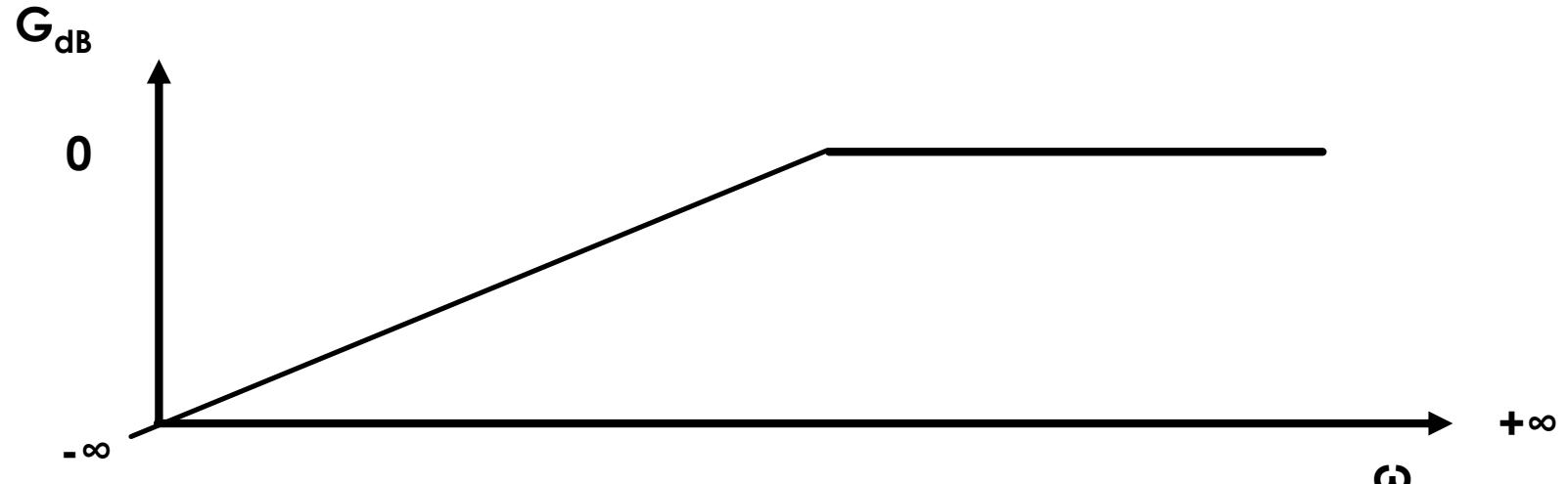
$$H_{PH}(j\omega) = A \frac{\left(j \frac{\omega}{\omega_0}\right)^2}{1 + 2mj \frac{\omega}{\omega_0} + \left(j \frac{\omega}{\omega_0}\right)^2}$$
