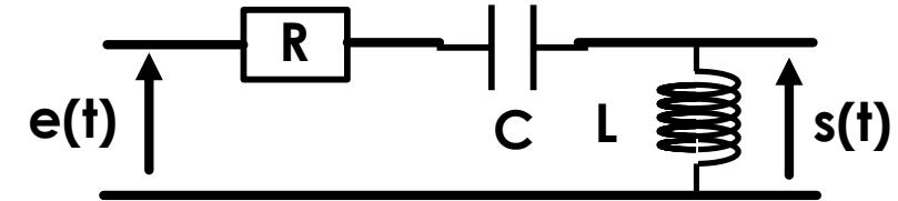
$$G_{dB}(\omega) = 40 \log_{10} \left( \frac{\omega}{\omega_0} \right) - 10 \log_{10} \left( 1 + (4m^2 - 2) \left( \frac{\omega}{\omega_0} \right)^2 + \left( \frac{\omega}{\omega_0} \right)^4 \right)$$
