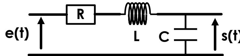
$$H_C(j\omega) = \frac{1}{1 + 2mj\frac{\omega}{\omega_0} + \left(j\frac{\omega}{\omega_0}\right)^2}$$
