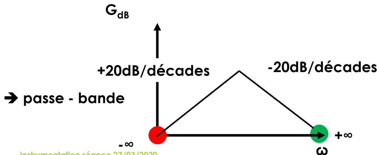
$$\Phi(\omega) = \frac{\pi}{2} - \arctan \left( \frac{2m}{\frac{\omega_0}{\omega} - \frac{\omega}{\omega_0}} \right)$$
