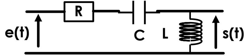
$$G(\omega) = \frac{\left(\frac{\omega}{\omega_0}\right)^2}{\sqrt{1 + (4m^2 - 2)\left(\frac{\omega}{\omega_0}\right)^2 + \left(\frac{\omega}{\omega_0}\right)^4}}$$
