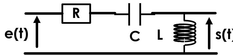
$$H_L(j\omega) = \frac{\left(j\frac{\omega}{\omega_0}\right)^2}{1 + 2mj\frac{\omega}{\omega_0} + \left(j\frac{\omega}{\omega_0}\right)^2}$$
