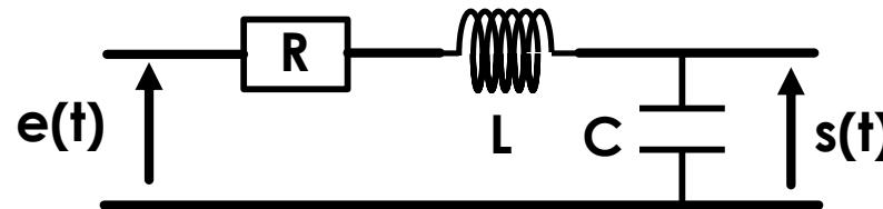
$$H_C(j\omega) = \frac{1}{1 + 2mj\frac{\omega}{\omega_0} + \left(j\frac{\omega}{\omega_0}\right)^2}$$
