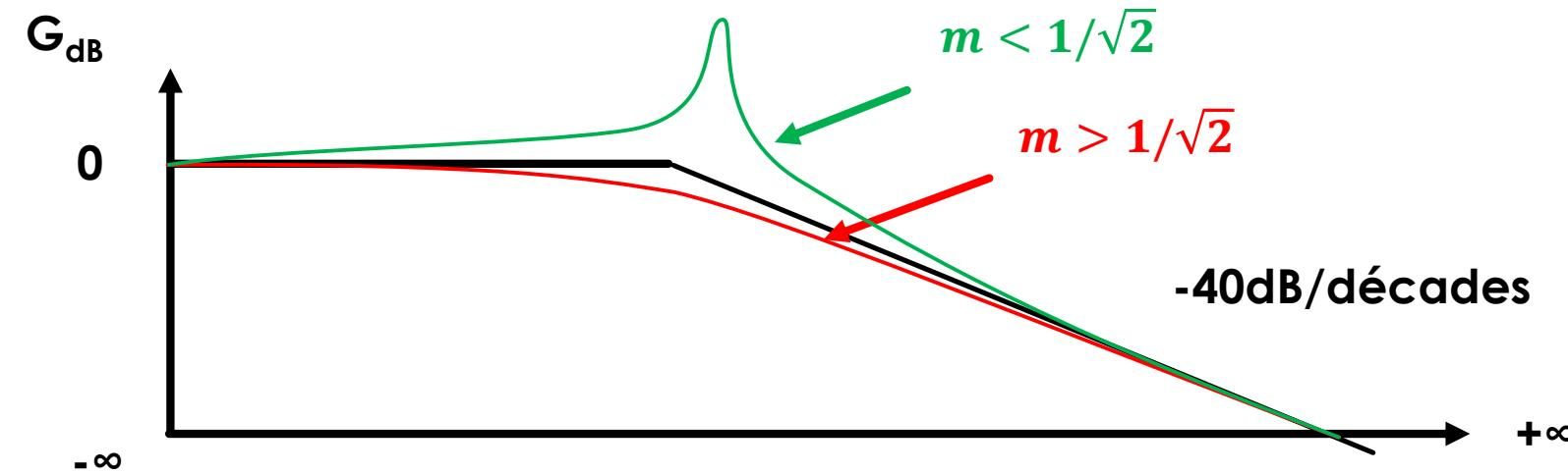
$$H_{PB}(j\omega) = A \frac{1}{1 + 2mj\frac{\omega}{\omega_0} + \left(j\frac{\omega}{\omega_0}\right)^2}$$
