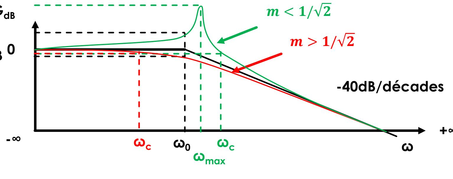
$$H_{PB}(j\omega) = A \frac{1}{1 + 2mj\frac{\omega}{\omega_0} + \left(j\frac{\omega}{\omega_0}\right)^2}$$
