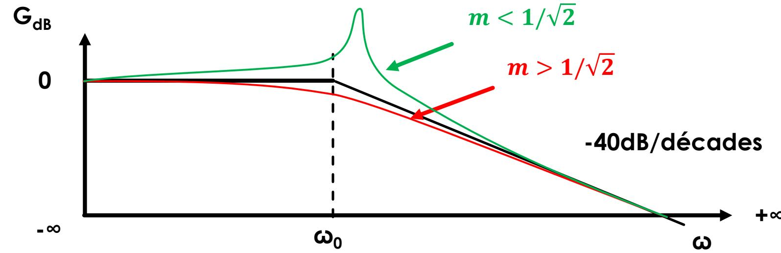
$$H_{PB}(j\omega) = A \frac{1}{1 + 2mj\frac{\omega}{\omega_0} + \left(j\frac{\omega}{\omega_0}\right)^2}$$
