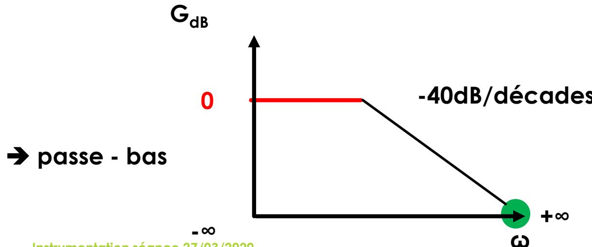
$$\Phi(\omega) = -\arctan \left( \frac{2m}{\frac{\omega_0}{\omega} - \frac{\omega}{\omega_0}} \right)$$
