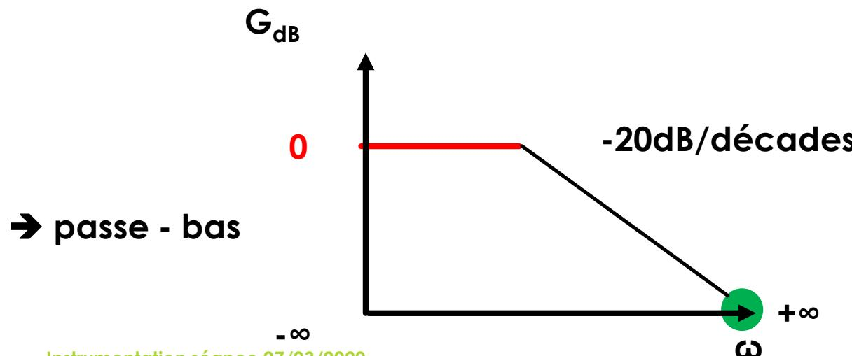
$$\Phi(\omega) = -\arctan \left( \frac{\omega}{\omega_0} \right)$$
