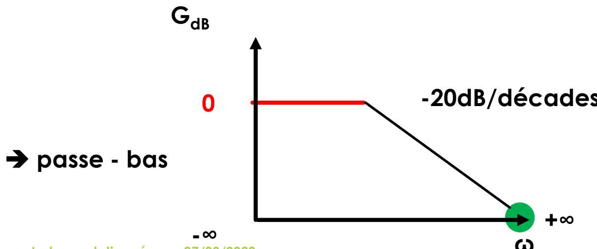
$$\Phi(\omega) = - \arctan \left( \frac{\omega}{\omega_0} \right)$$
