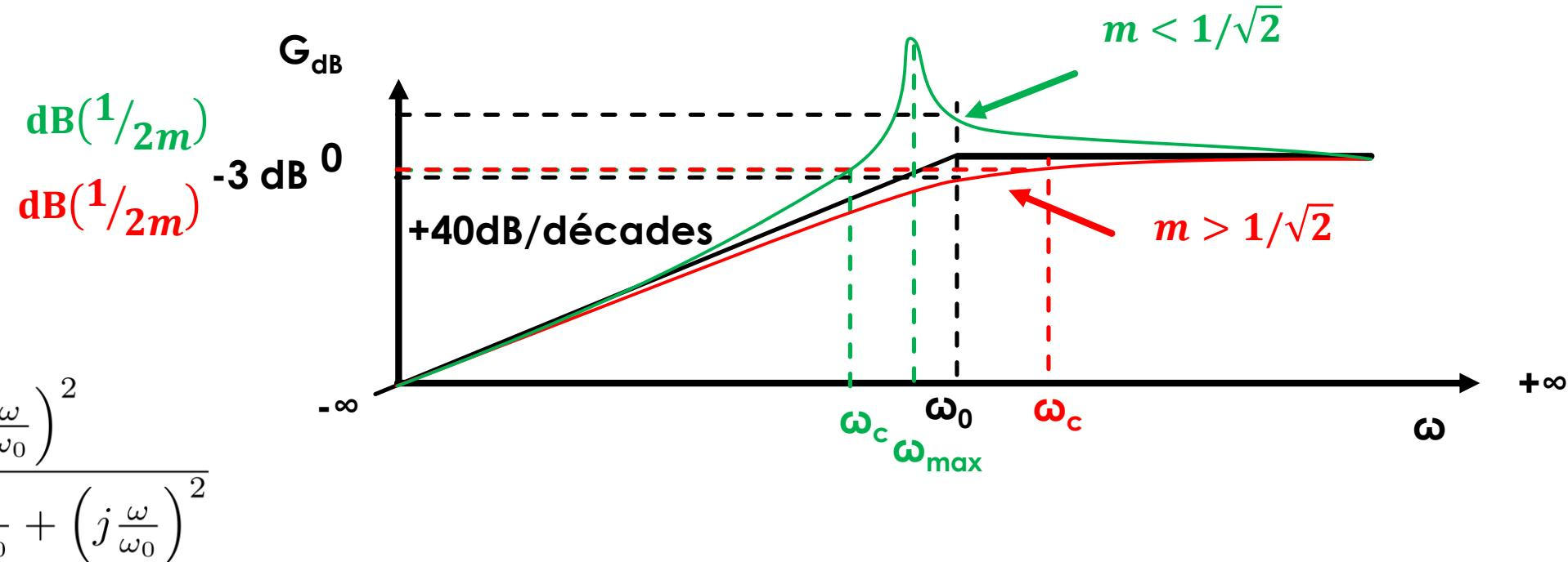
$$H_{PH}(j\omega) = A \frac{\left(j \frac{\omega}{\omega_0}\right)^2}{1 + 2mj \frac{\omega}{\omega_0} + \left(j \frac{\omega}{\omega_0}\right)^2}$$
