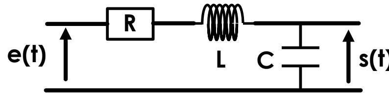
$$H_C(j\omega) = \frac{1}{1 + 2mj\frac{\omega}{\omega_0} + \left(j\frac{\omega}{\omega_0}\right)^2}$$
