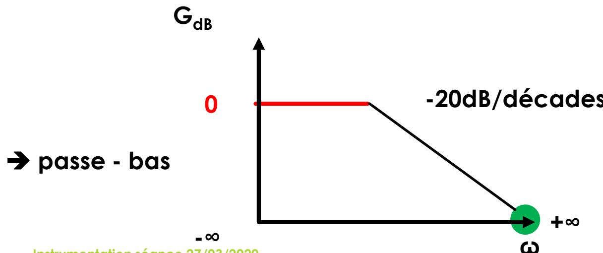
$$\Phi(\omega) = -\arctan \left( \frac{\omega}{\omega_0} \right)$$
