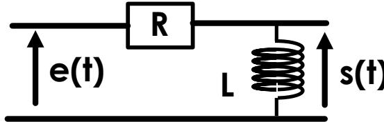
$$H(j\omega) = \frac{S(\omega)}{E(\omega)} = H_1 \times H_2 = \frac{j \frac{\omega}{\omega_0}}{1 + j \frac{\omega}{\omega_0}}$$
