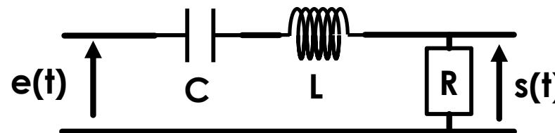
$$H_R(j\omega) = \frac{2mj\frac{\omega}{\omega_0}}{1 + 2mj\frac{\omega}{\omega_0} + \left(j\frac{\omega}{\omega_0}\right)^2}$$
