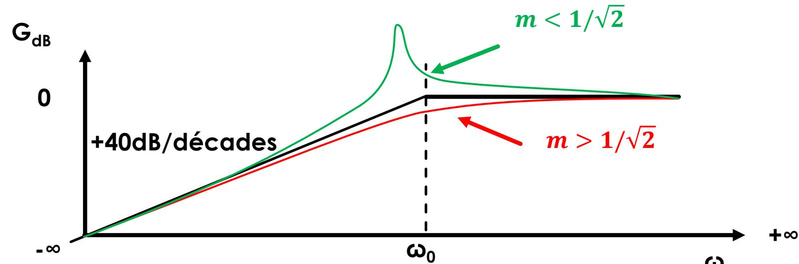
$$H_{PH}(j\omega) = A \frac{\left(j \frac{\omega}{\omega_0}\right)^2}{1 + 2mj \frac{\omega}{\omega_0} + \left(j \frac{\omega}{\omega_0}\right)^2}$$
