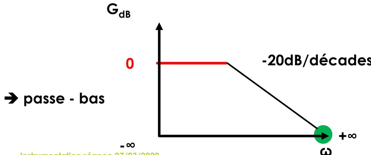
$$\Phi(\omega) = -\arctan \left( \frac{\omega}{\omega_0} \right)$$
