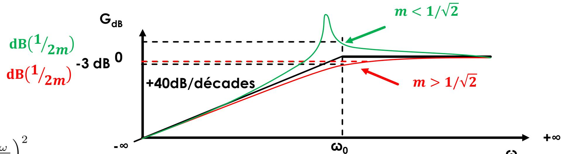
$$H_{PH}(j\omega) = A \frac{\left(j \frac{\omega}{\omega_0}\right)^2}{1 + 2mj \frac{\omega}{\omega_0} + \left(j \frac{\omega}{\omega_0}\right)^2}$$
