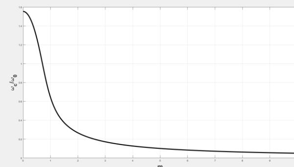
$$G(\omega) = \frac{1}{\sqrt{1 + (4m^2 - 2) \left(\frac{\omega}{\omega_0}\right)^2 + \left(\frac{\omega}{\omega_0}\right)^4}}$$
