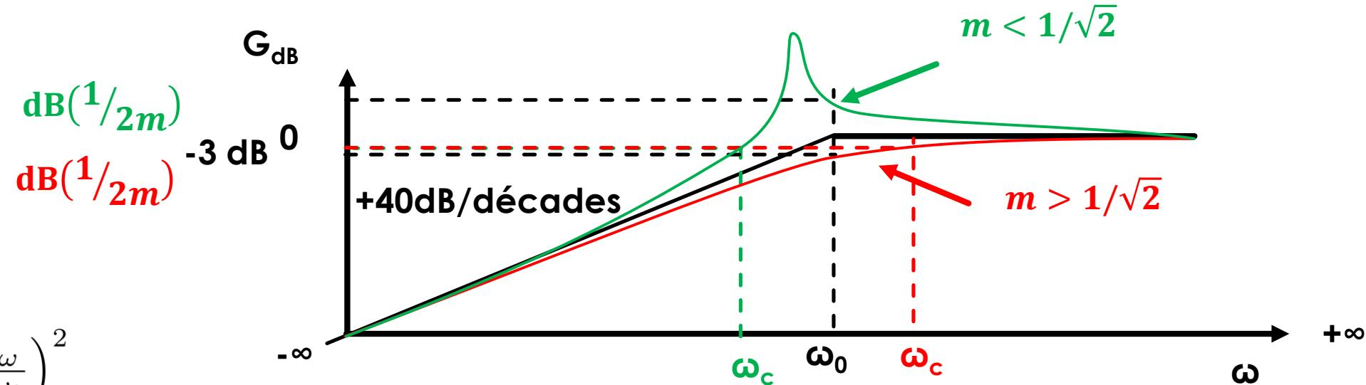
$$H_{PH}(j\omega) = A \frac{\left(j \frac{\omega}{\omega_0}\right)^2}{1 + 2mj \frac{\omega}{\omega_0} + \left(j \frac{\omega}{\omega_0}\right)^2}$$
