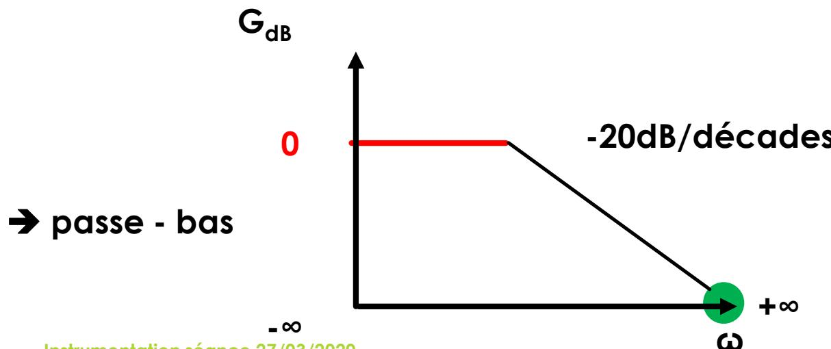
$$\Phi(\omega) = -\arctan \left( \frac{\omega}{\omega_0} \right)$$
