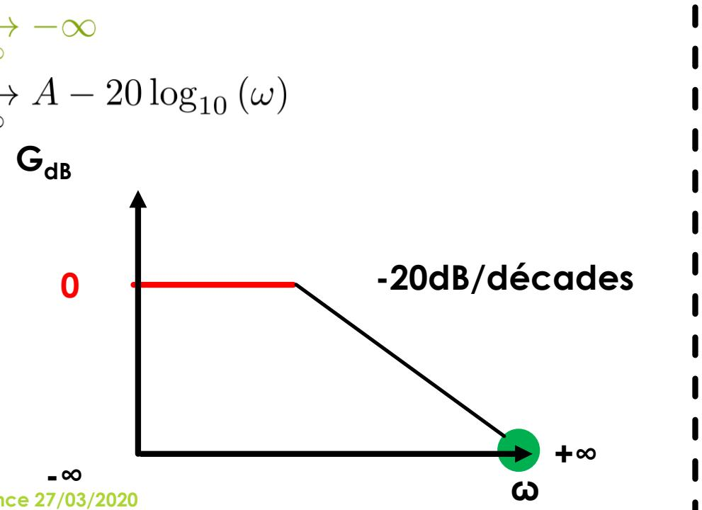
$$\Phi(\omega) = -\arctan \left( \frac{\omega}{\omega_0} \right)$$
