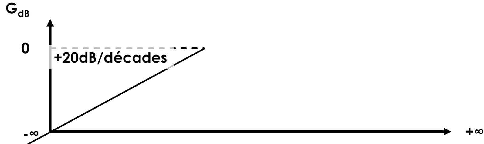
$$H_{PBand}(j\omega) = A \frac{2mj\frac{\omega}{\omega_0}}{1 + 2mj\frac{\omega}{\omega_0} + \left(j\frac{\omega}{\omega_0}\right)^2}$$
