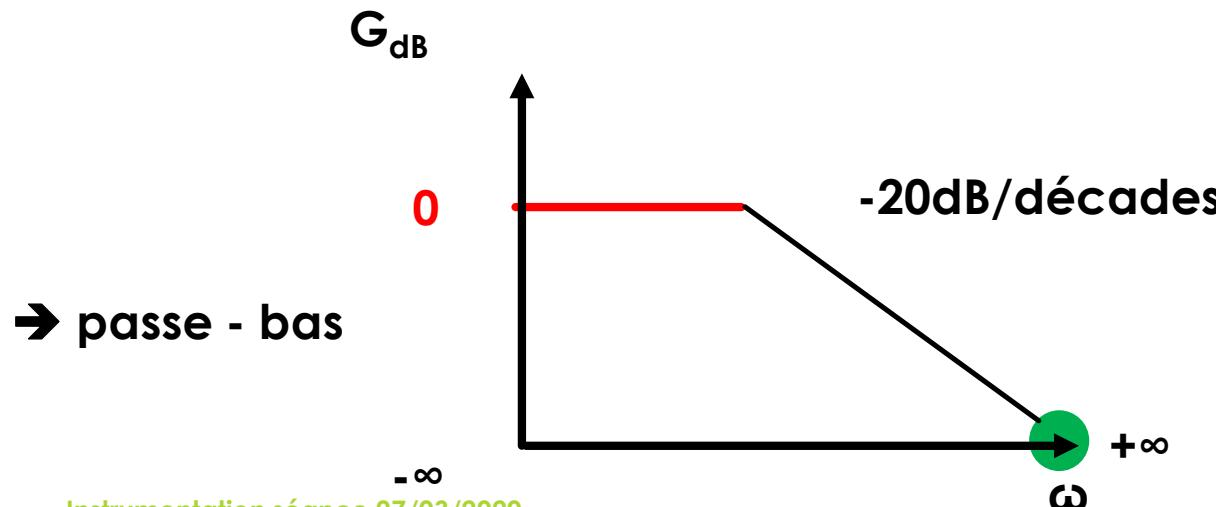
$$\Phi(\omega) = -\arctan \left( \frac{\omega}{\omega_0} \right)$$
