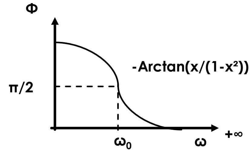
$$G_{dB}(\omega) = 40 \log_{10} \left( \frac{\omega}{\omega_0} \right) - 10 \log_{10} \left( 1 + (4m^2 - 2) \left( \frac{\omega}{\omega_0} \right)^2 + \left( \frac{\omega}{\omega_0} \right)^4 \right)$$
