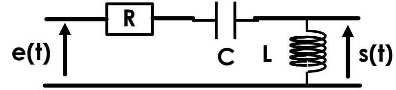
$$G(\omega) = \frac{\left(\frac{\omega}{\omega_0}\right)^2}{\sqrt{1 + (4m^2 - 2)\left(\frac{\omega}{\omega_0}\right)^2 + \left(\frac{\omega}{\omega_0}\right)^4}}$$
