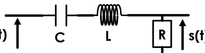
$$\Phi(\omega) = \frac{\pi}{2} - \arctan \left( \frac{2m}{\frac{\omega_0}{\omega} - \frac{\omega}{\omega_0}} \right)$$
