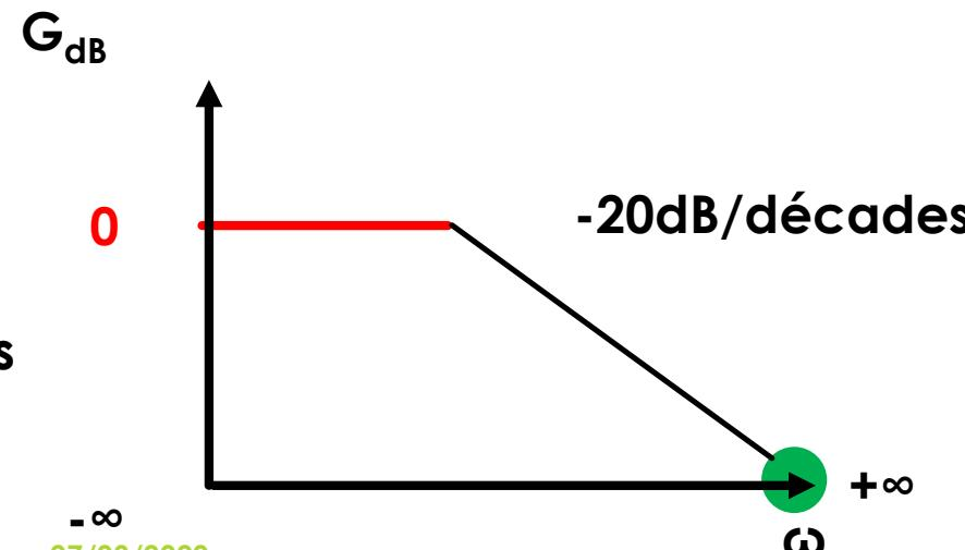
$$\Phi(\omega) = - \arctan \left( \frac{\omega}{\omega_0} \right)$$
