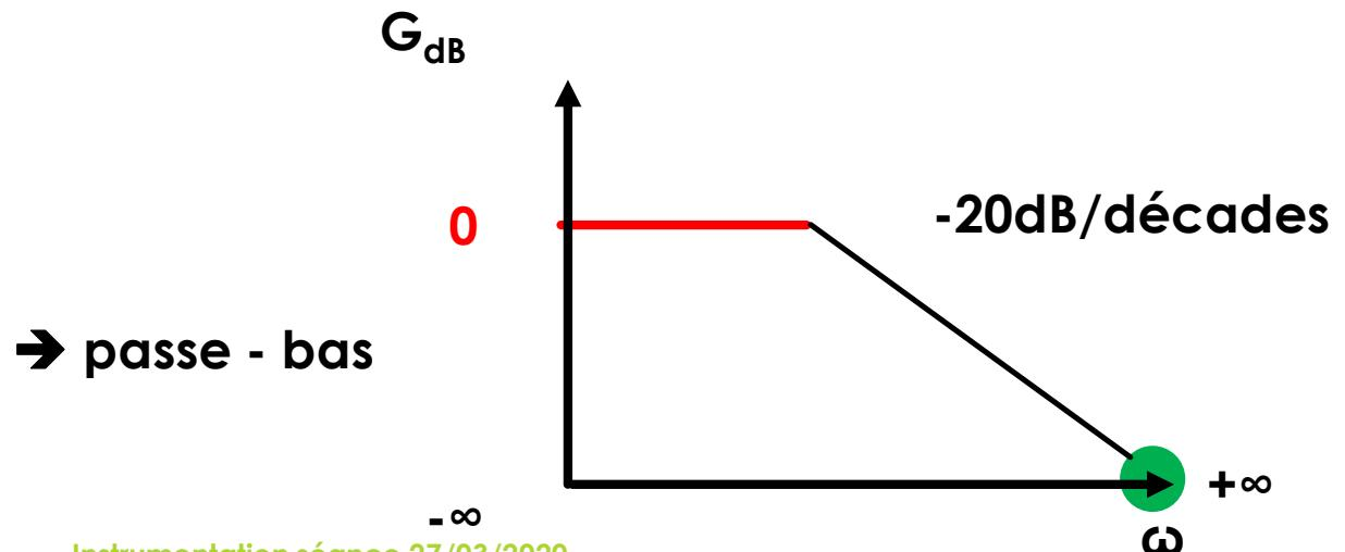
$$\Phi(\omega) = -\arctan \left( \frac{\omega}{\omega_0} \right)$$
