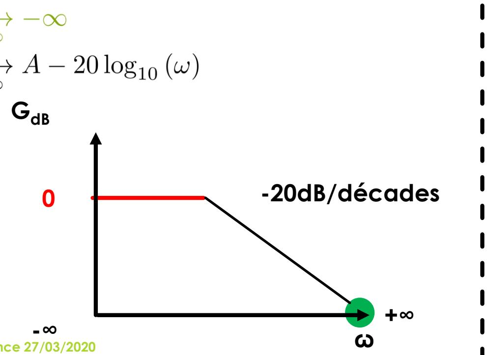
$$\Phi(\omega) = -\arctan \left( \frac{\omega}{\omega_0} \right)$$
