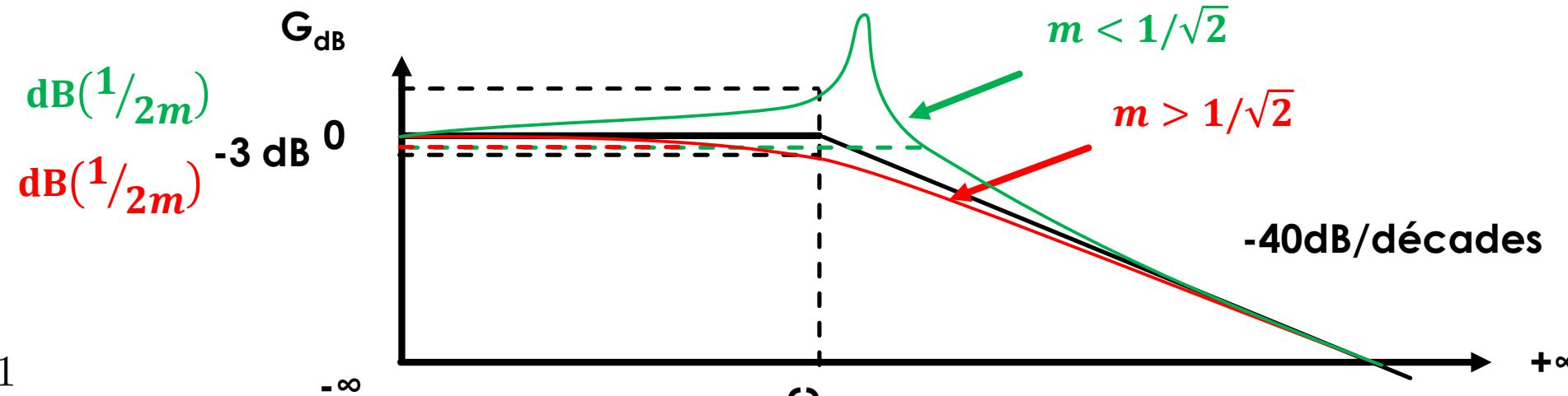
$$H_{PB}(j\omega) = A \frac{1}{1 + 2mj\frac{\omega}{\omega_0} + \left(j\frac{\omega}{\omega_0}\right)^2}$$
