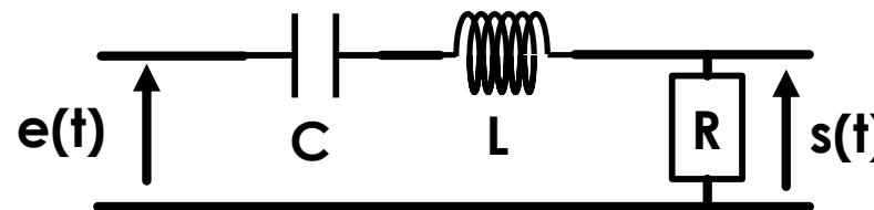
$$H_R(j\omega) = \frac{2mj\frac{\omega}{\omega_0}}{1 + 2mj\frac{\omega}{\omega_0} + \left(j\frac{\omega}{\omega_0}\right)^2}$$
