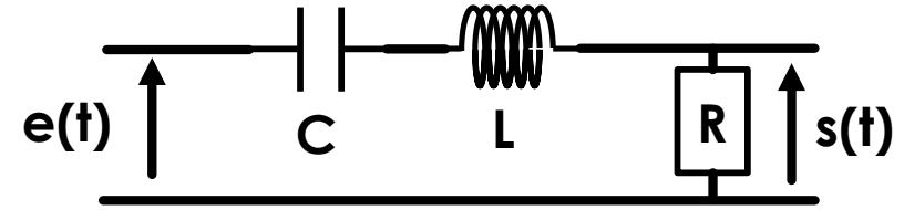
$$G(\omega) = \frac{2m \frac{\omega}{\omega_0}}{\sqrt{1 + (4m^2 - 2) \left(\frac{\omega}{\omega_0}\right)^2 + \left(\frac{\omega}{\omega_0}\right)^4}}$$
