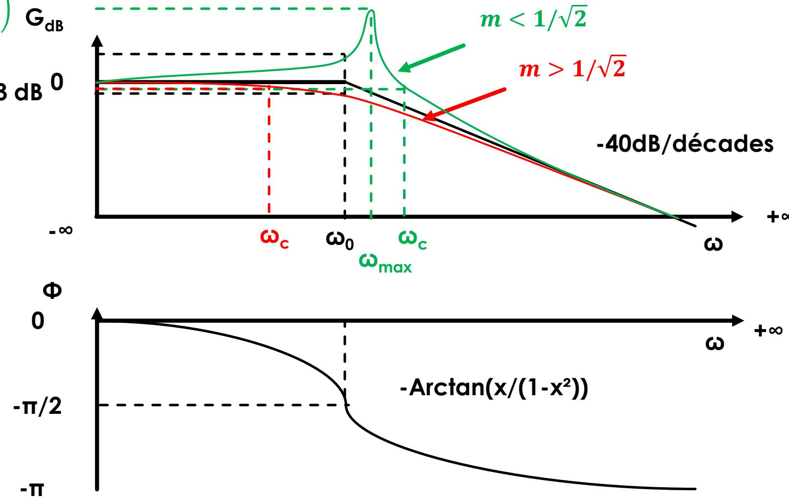
$$H_{PB}(j\omega) = A \frac{1}{1 + 2mj\frac{\omega}{\omega_0} + \left(j\frac{\omega}{\omega_0}\right)^2}$$
