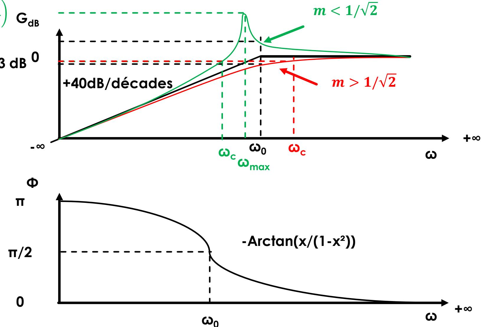
$$H_{PH}(j\omega) = A \frac{\left(j\frac{\omega}{\omega_0}\right)^2}{1 + 2mj\frac{\omega}{\omega_0} + \left(j\frac{\omega}{\omega_0}\right)^2}$$
