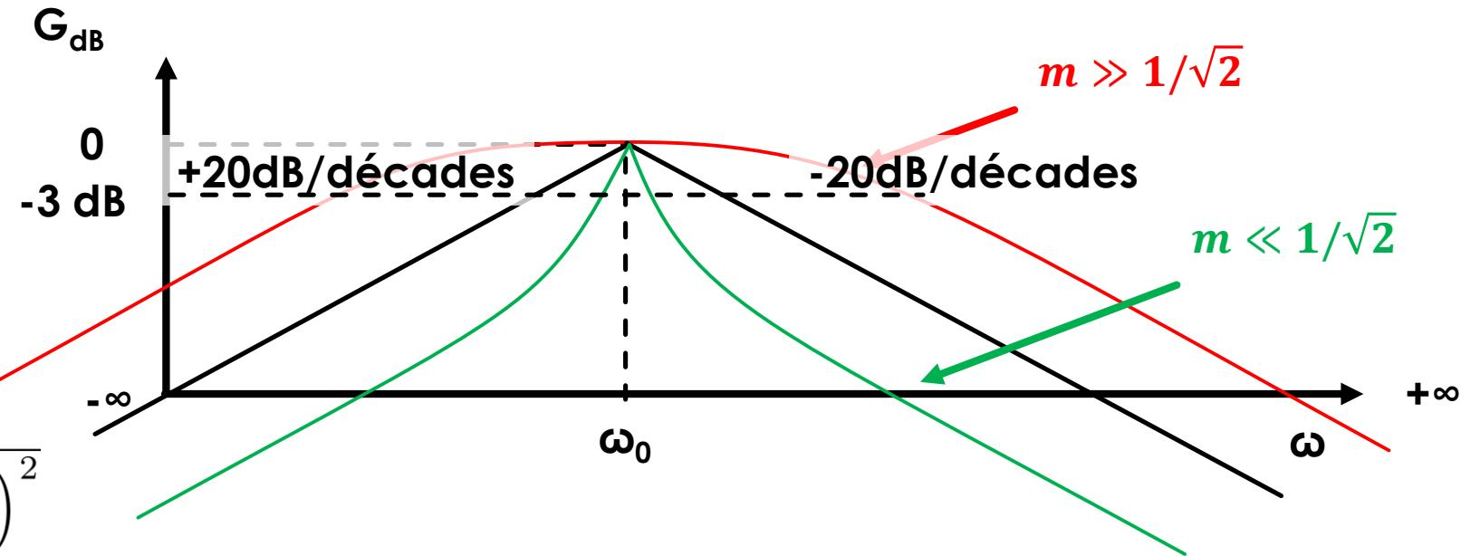
$$H_{PBand}(j\omega) = A \frac{2mj \frac{\omega}{\omega_0}}{1 + 2mj \frac{\omega}{\omega_0} + \left(j \frac{\omega}{\omega_0}\right)^2}$$
