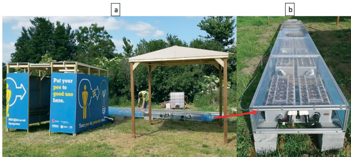
Fig. 2 (a) Pee power field trial in Glastonbury Music Festival, June 2015; (b) urinal assembly and MFC stack arranged in 12 modules.
