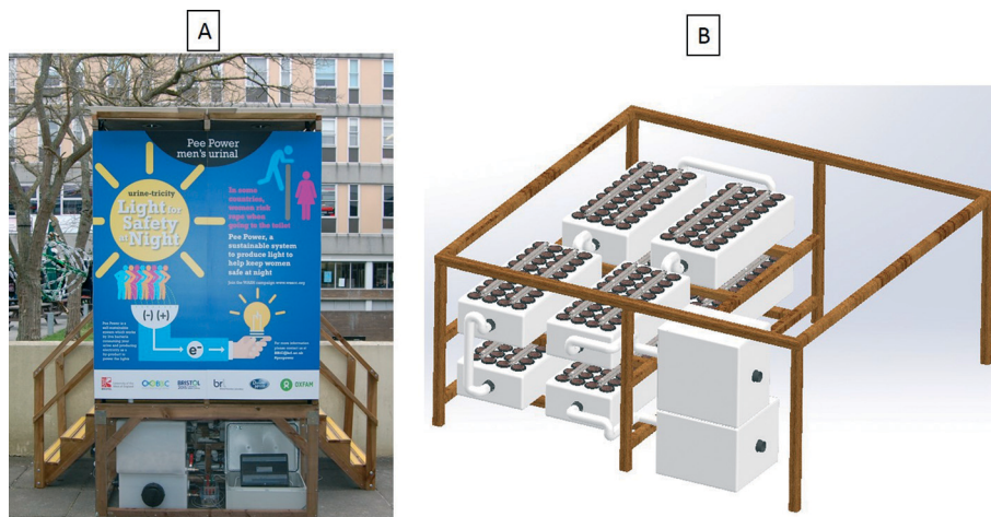
Fig. 1 (A) Pee power field trial funded by Oxfam at the UWE campus in February–May 2015; (B) 3D representation of the MFC stack with the inlet and outlet tanks underneath the urinal.
