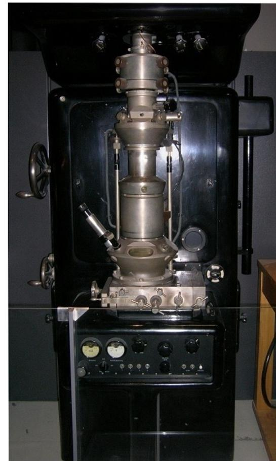
*Image: Replica from 1980 by Ernst Ruska of the first electron microscope with resolving power higher than that of a light microscope made by Ernst Ruska 1933. ©J Brew/ commons.wikimedia.org. Shared under: Creative Commons License.*
