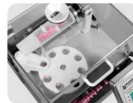
Test specimens can be weighed quickly and accurately with the CW automatic weighing system
