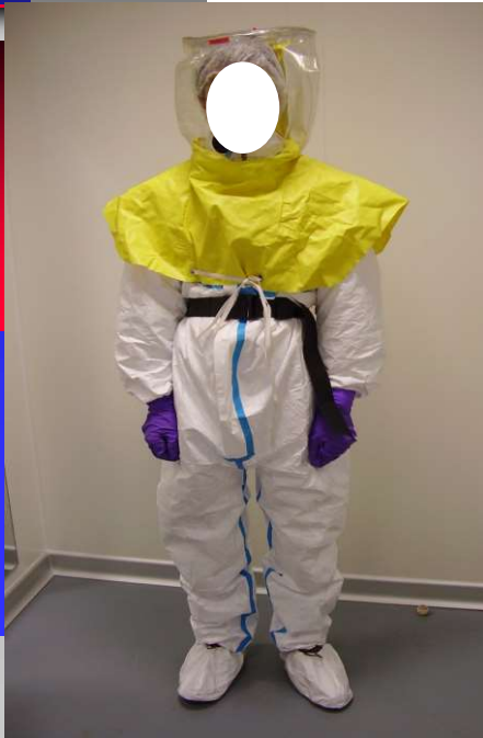
Ventilated hood Containment level : 100 \mu\text{g}/\text{m}^3 (8h TWA)
