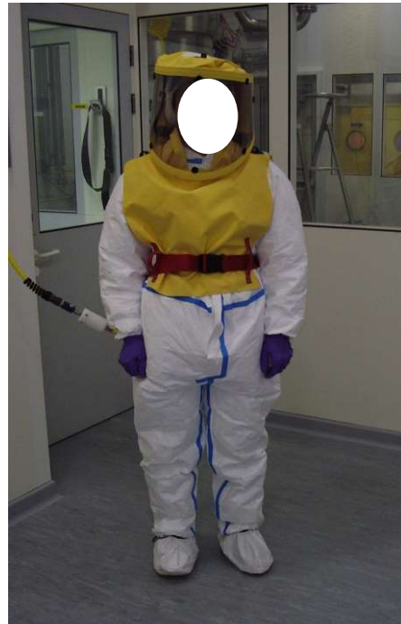
Hood with breathable air Containment level : 100 \mu\text{g}/\text{m}^3 (8h TWA) Use of N2
