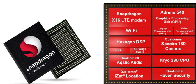
Figure 1.4: SoC Qualcomm Snapdragon 835: more than 3 billion transistors. It contains a GPU, DSP, modem LTE, audio codec, camera ISP and a CPU Qualcomm Kryo 280 (8 cores, 4 x 2.45 GHz with 2MB cache L2 + 4 x 1.9 GHz with 1MB cache L2).
