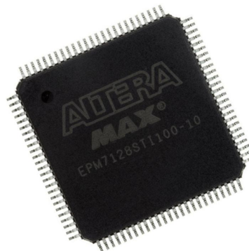
Figure 1.18: CPLD EPM7128S MAX 7000 from Altera includes CMOS EEPROM cells, 2500 logic gates, 128 macro-cells, 8 LAB and 100 I/O. Each LAB is formed by 16 macro-cells.
