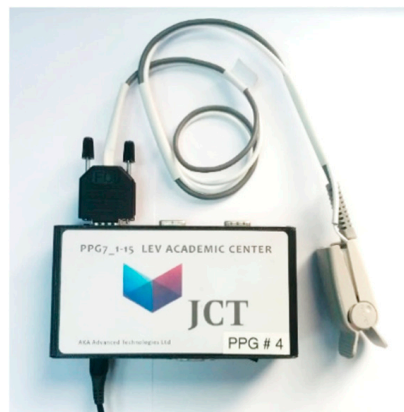
Figure 4. The control unit of the JCT pulse oximeter device together with an adult finger probe.
