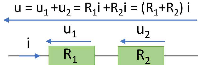
$$u_1 = R_1 i \text{ et } u = (R_1 + R_2) * i \text{ donc } u_1 = \frac{R_1}{R_1 + R_2} u$$
