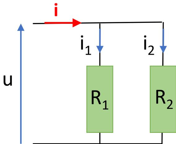
$$i_1 = u/R_1 \text{ et } i = (1/R_1 + 1/R_2) * u \text{ donc } i_1 = \frac{\frac{1}{R_1}}{\frac{1}{R_1} + \frac{1}{R_2}} i = \frac{R_2}{R_1 + R_2} i$$
