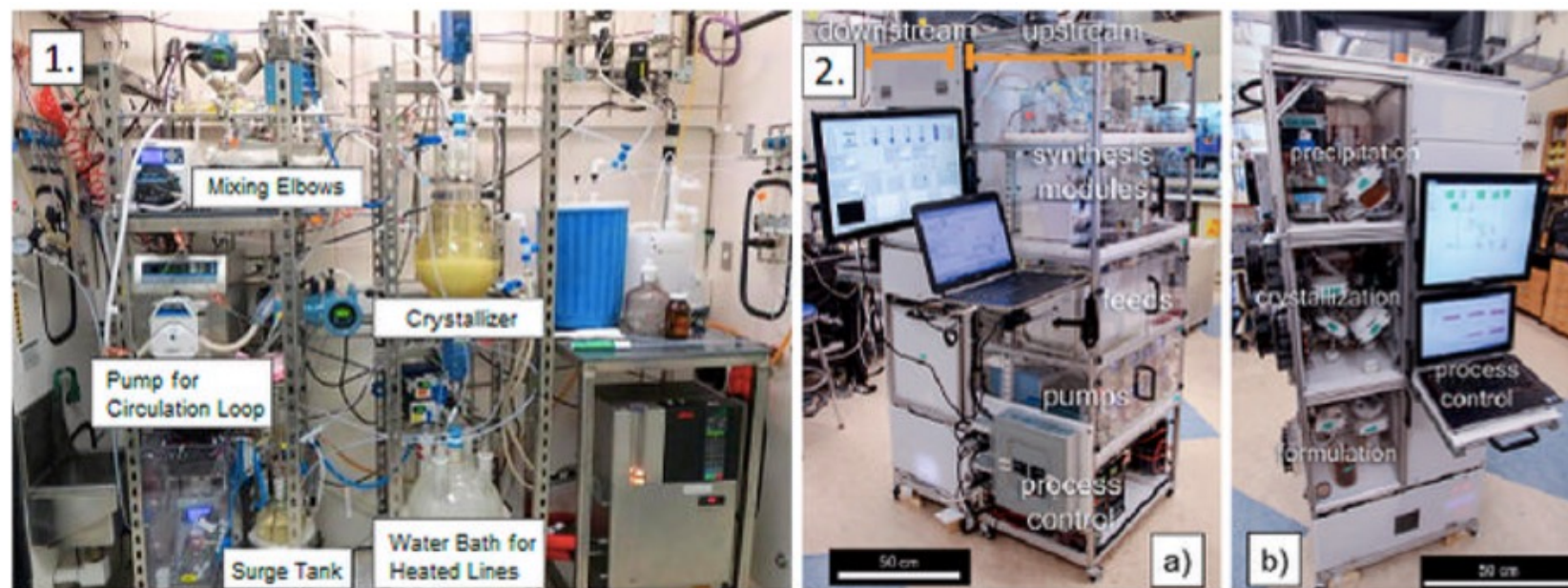
Figure 3. A system operated in a fume hood for continuous API production. (1) A pilot-scale continuous system for the production of LY2886721. Adapted with permission from ref 85. Copyright 2020 American Chemical Society. (2) (a) Upstream and (b) downstream units for continuous on-demand production of API. From ref 86. Reprinted with permission from AAAS.
