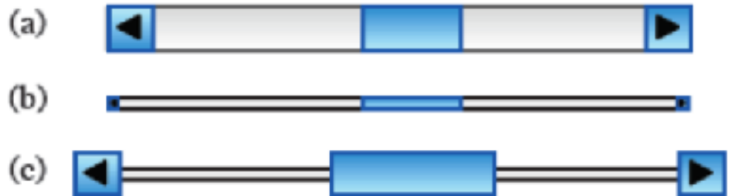
Figure 12: Scroll-bar redesign (a) original version. (b) new version: visual space (what it looks like) and (c) motor space (what it feels like when interacting with it).
