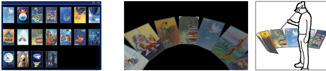
Figure 2: Different virtual surfaces. On the left, an image of a typical virtual Surface with CARDS. On the middle and right, views of the Personal Space : first, a view from the user’s headset, with CARDS organized in a belt configuration that follows the user; and next, a rendering that highlights the relative position and size of the belt with respect to the user.
