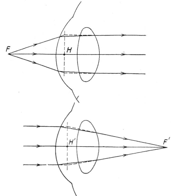
$$\left\{ \begin{array}{l} f' = \frac{1,33}{1,33 - 1} \times 5,6 \text{ mm} = 22,3 \text{ mm} \\ f = -\frac{1}{1,33 - 1} \times 5,6 \text{ mm} = 16,7 \text{ mm} \end{array} \right. \implies P_{\text{oeil}} = \frac{1,33}{0,0223} = 60 \text{ m}^{-1}(\delta)$$
