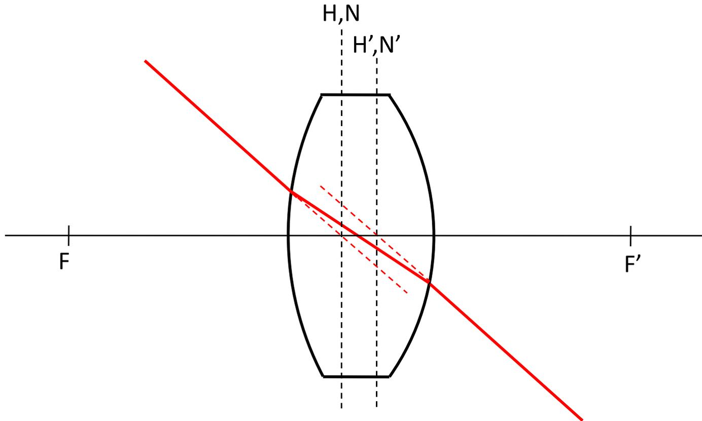
$$\frac{1}{\overline{H'F'}} = (n - 1) \left( \frac{1}{\overline{S_1C_1}} - \frac{1}{\overline{S_2C_2}} \right) + \frac{(n - 1)^2}{n} \frac{\overline{S_1S_2}}{\overline{S_1C_1} \times \overline{S_2C_2}}$$
