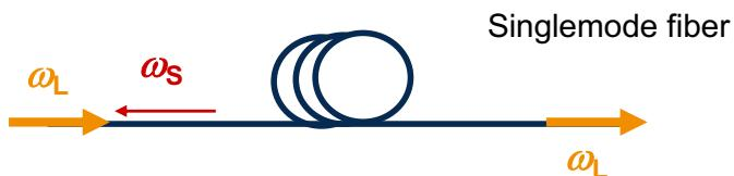
Calculation of the number of Stokes photons created through the amplification of the photons initially created through spontaneous Brillouin scattering
