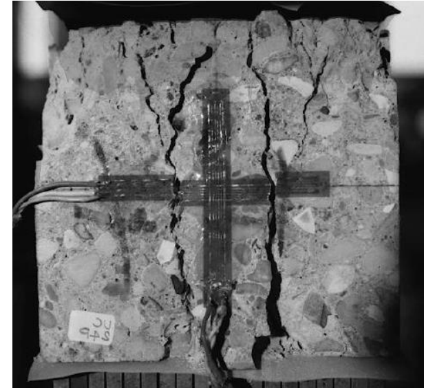
Rupture sans frettage
