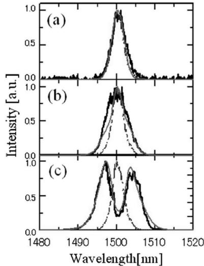
FIG. 1 – Output spectra measured at the waveguide output for injected powers respectively equal to (a) 0.13 W, (b) 1.02 W and (c) 2.05 W.
